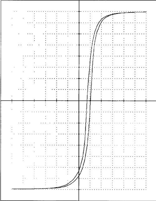
The final example to the left is referred to as a Delta P plot. This plots the relationship between pressure drop across the valve and flow rate achieved. This plot does not always accompany all valve repair documentation.
