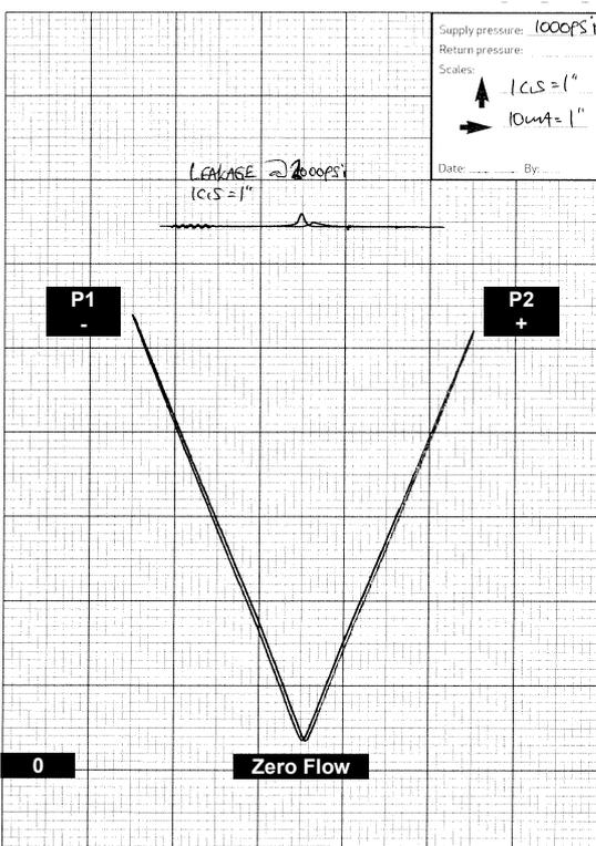
This type of plot differs from the usual expanded flow plot because the measurement of flow is taken in the return port.
