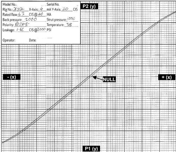
An expanded flow plot is the most common type which accompanies test data. This plot shows your servovalve flow performance and indicates other characteristics including Hysteresis, lap condition, and null bias.
